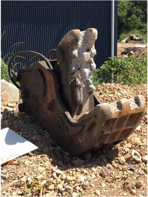
SQUEEZE MECHANISM ATTACHED TO EXCAVATOR
